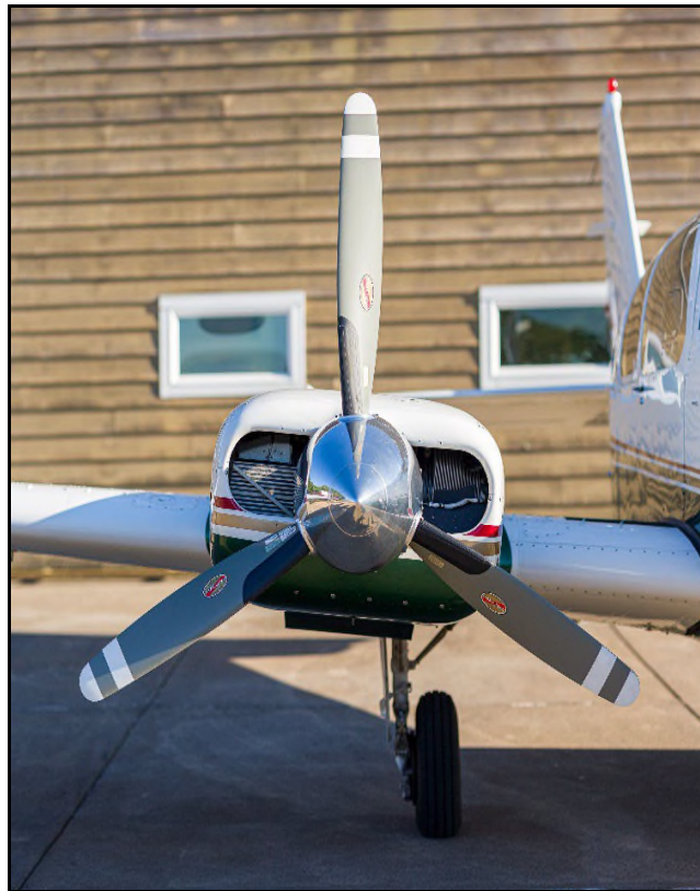
Left Photo: View of wheel, lights and landing gear. Note: 3 bladed propellers, new tire, clean joints and no oil leaks.
