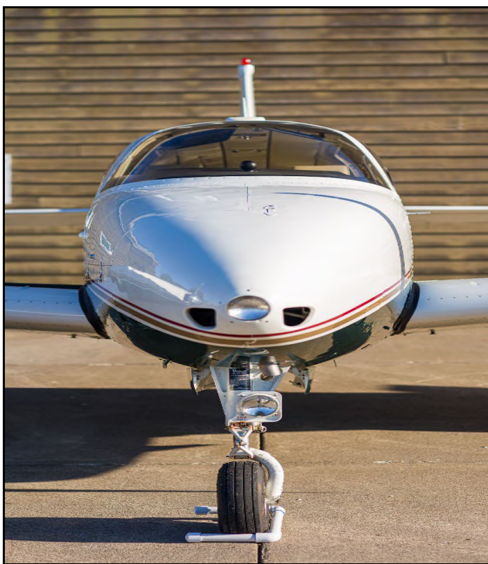
Left Photo: View of wheel, lights and landing gear. Note: 3 bladed propellers, new tire, clean joints and no oil leaks.
